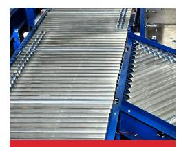
ITR Merge bed is designed to have a spur mounted to it. Adjustable speeds between 25 FPM to the maximum speed of 180 FPM.
